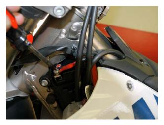
Max torque for the terminal screws is 30kg/cm (26 inch/pound). Do not over-tighten. We recommend the use of a #3 (big!) Phillips screwdriver, as this allows you to apply downward pressure on the terminal screw. That helps the threads catch, and reduces torque on the terminals. Note that the terminals are not anchored at back, and may twist slightly during install. If so, performance is not affected.
